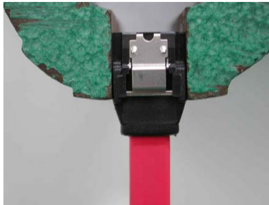
Fig. 2 : Hold the near end of the cable plug with a clamp
