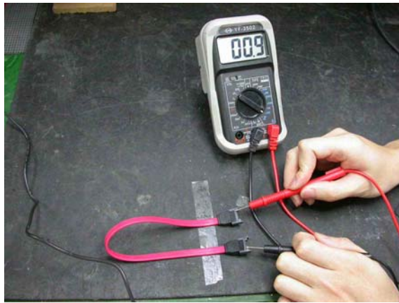
Fig. 4 : Conductor resistance measurement condition
